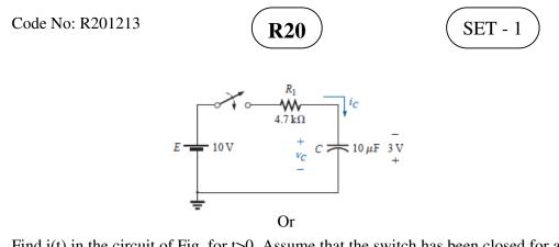
4 a) Find i(t) in the circuit of Fig. for t>0. Assume that the switch has been closed for a (7M) long time.
