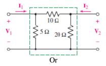
10 a) Find the impedance parameters for the two-port shown in Fig.
