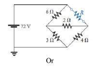
8 a) Find the Thevenin equivalent circuit for the bridge network across the terminals (7M) a&b. Also find the current through the resistor of 1  $\Omega$  connected between a &b?
