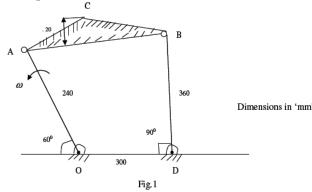
A shaper mechanism is shown in figure. The crank OA rotates at uniform speed of (14M)
