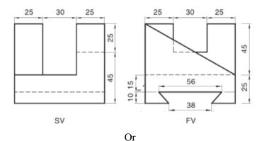
Draw the elevation, plan and left side view of the object given below. (14M)
